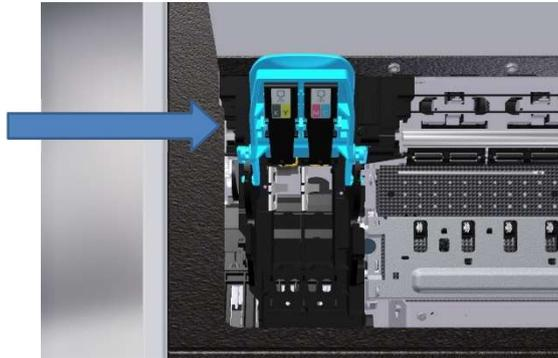
Insert the two printheads into its color-coded slot. „KY for black-yellow and MC for magenta-cyan“
