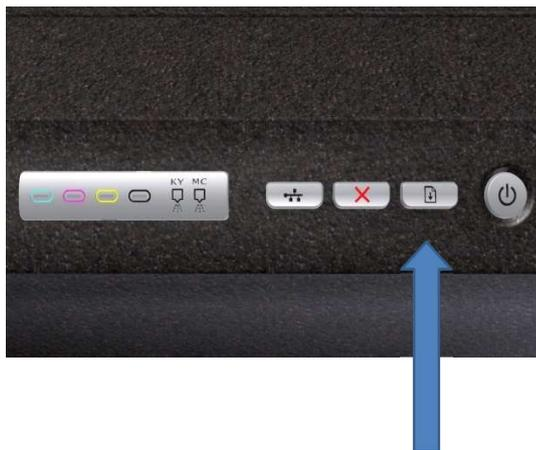
Until the carriage moves to the left, wait for the carriage stop moving.
