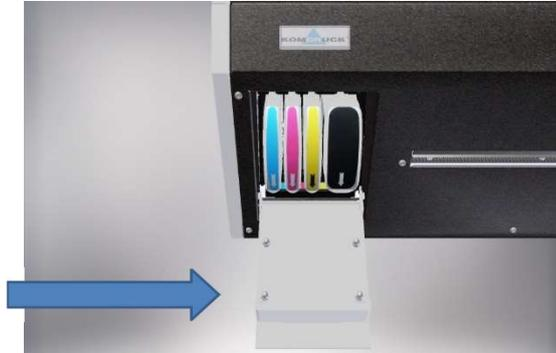
Align the cartridge with its color-coded slot and insert the cartridge into the slot. The directional arrow down face down. Press down firmly on the cartridge to ensure proper contact.
