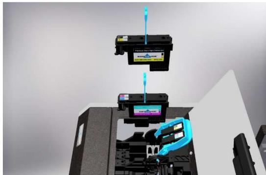
Fold the printhead latch down and close the cover.
